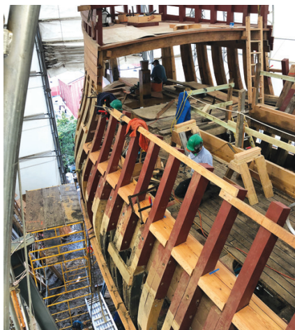
Clockwise from top left: Mystic Seaport shipwrights Brett Land drilling holes for trunnels, Anthony Daniels fairing the hull, Greg See installing waterways, and Anthony Matt hand-planing a plank.
