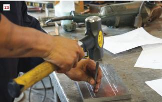
The steps for basic metal-shop work are set by standards to ensure consistent work throughout the industry. Here, a fabricator follows the standard procedures for laying out bolt-hole positions (12) and marking them with a center punch (13).
