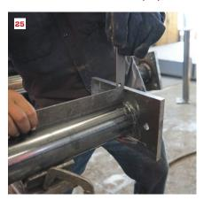
With the plate positioned at the layout marks, the fabricator tack welds the plate to the column in four places. Before completing the weld, he makes sure the plate is square to the column on one side (24), then he flips the column to check the other side (25).
