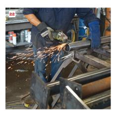
Most residential steel welding is done in the fabrication shop with a MIG welder (20). Welding a connection plate onto a column starts with checking the cut for square (21). The fabricator then cleans the end of the column with an abrasive wheel (22).
