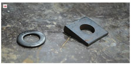
Torsion control (TC) bolts maintain specific torque settings. After threading on the nut (16), a special wrench tightens it while gripping the splined end (17), which breaks off at a given torque (18). Washers should always be made from hardened steel (19).
