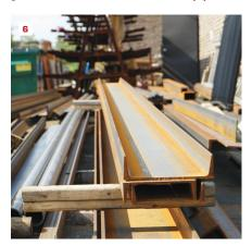
Engineers often specify steel I-beams to carry heavy loads or to span large distances in a home (4). On plans, beams are labeled according to size and weight (5). Steel channel is often specified for support instead of I-beams (6).
