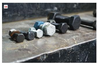
Bolts for residential steel work should all have an ASTM number stamped on the head, which means that they have a specific strength rating. A307 is a non-high strength bolt (14), while A325 may be specified for high-strength applications (15).
