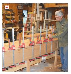
Each face of the column butts on one side and laps over the other. After routing the panel pattern into a few sides, the author assembled them in pairs, running a bead of glue down the edge of one side (8). To hold the two adjacent sides in alignment, he tacked them together with brads (9), then he fully clamped the assembly and moved on to the next pair of panels while waiting for the glue to set (10). After removing the clamps, the author cleaned up the joints with a belt sander.
