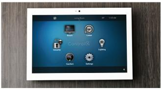
Mandalay Homes' basic workforce housing includes a programmable, internet-capable thermostat supplied by Trane (top). But in most houses, a Control4 home automation interface takes over the job of the thermostat. This Control4 panel also manages lighting, audio, video, and more (above).
