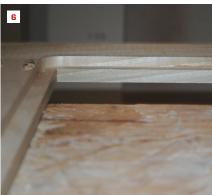
Two routers are fitted with different bits (3) to cut the rabbets for the plywood panels (4). The first pass, done with the bit with the large bearing, makes a shallow cut and leaves a clean edge (5). On the second pass, the router bit with the smaller bearing finishes the rabbet, hogging out the material to the full width of the rabbet (6).
