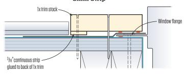
To keep flat stock trim in plane with the wall while creating a place for the siding to die into, either rabbet thicker trim over the flange or hold 1-by stock off the wall with a shim strip or stand-off screws.
