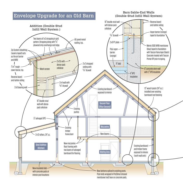
In order to accomplish a well-insulated airtight envelope on a tight budget, Maine Passive House relied on a combination of advanced membranes and recycled existing materials. Existing barnboard was left exposed on the roof underside and on one wall. The built-up I-joist roof system above the existing timbers is completely enclosed in vapor management membranes.
