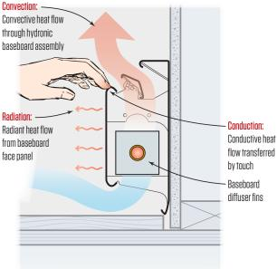
Heat flows from warm to cold. In a framed wall assembly, cavity insulation limits conductive heat flow, but the studs themselves can also transfer heat through the assembly unless continuous insulation, such as rigid foam, is installed (above left). A fin-tube radiator (above right) transfers little heat by radiation. It mostly moves heat by convection (air flowing through the diffuser fins) and by conduction (heat moving across the pipe wall and into the aluminum fins).
