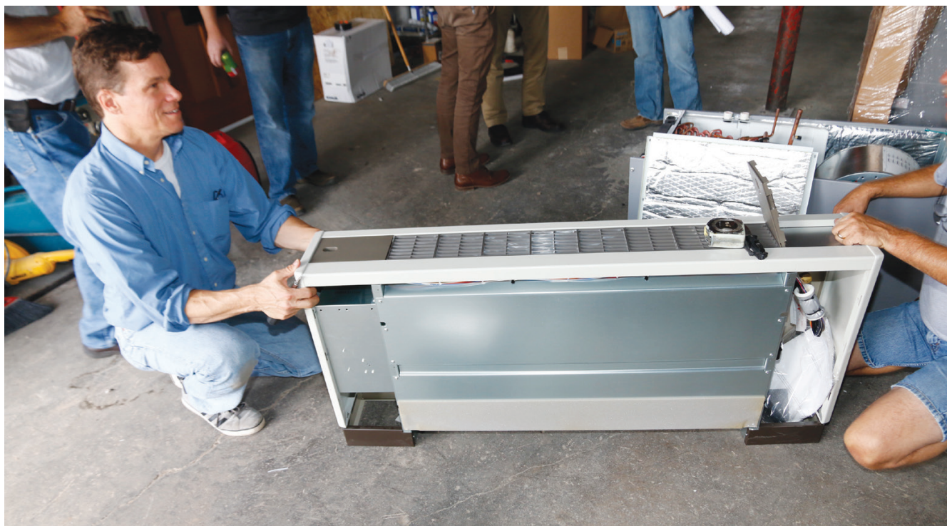
The author examines a Mitsubishi PFFY compact air handler. This small unit is useful for handling the heating and cooling requirements of peripheral zones in a building and can be one of multiple air-handling units connected to the same outdoor VRF compressor.
