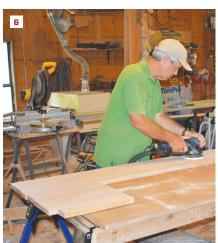
For the step blanks, the author glued up oak strips, alternating the growth rings up and down between pieces (1). He added a piece for the final width of the bottom step (2). The upper step was not as wide (3), and he planed the blank in one shot (4). The last blank consisted of  $\frac{3}{4}$ -inch oak strips with a  $\frac{5}{4}$ -inch bullnose strip (5). Finally, the blanks were rough sanded (6).
