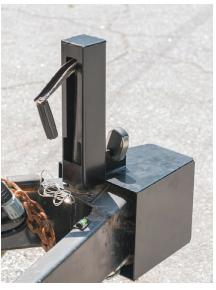
The Vault isolates the tongue and the crank (jackstand handle) from tampering and from the power tools or bolt cutters of would-be thieves.
