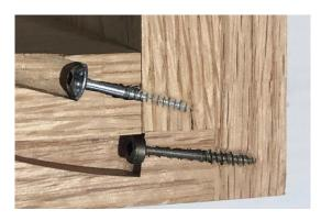
The TSM-12 bores a lower-angle (6 degrees) pocket (bottom, in photo) than other jigs (15 degrees, top, in photo). This enables the screw to bite into the receiver stock with a decreased tendency to shift that stock out of place.
