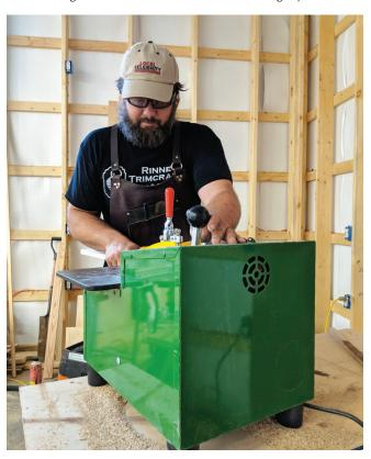
The TSM-12 includes a Bosch 1617 Router, Bosch Colt Router, <sup>9</sup>/<sub>64</sub>-inch premium drill bit, and <sup>3</sup>/<sub>8</sub>-inch three-flute solid carbide router bit. While you can use other brands of pockethole screws, Castle also sells them (not included).
