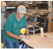
Using the arc as a form, the author glued up strips for the nosing (7). After planing the nosing (8), he glued it to the tread (9) and routed a bullnose on the edge (10).
