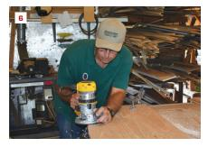
After attaching a router to a 1x6 trammel board set at the proper radius, the author cut a groove along the arc with a dado bit (4). He followed the groove with a jigsaw (5), then finished cutting the arc with a bearing-guided flush trim bit in the router (6).
