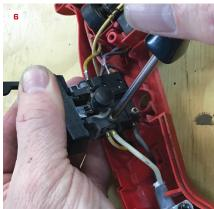
Before removing the wires, the author takes pictures of the switch and wires so he can make sure that he puts them back together properly. To remove the wires from the switch, he depresses springloaded metal keepers with a pick (5). On the opposite side of the switch, he backs off screws that hold the wires in place on that side (6).
