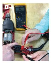
To access the switch, the author removes the screws holding the handle together (1), including one below the rubber grip (2). He then separates the halves of the handle (3). To confirm that the switch is bad, the author depresses the switch while a helper checks the continuity through the switch (4).
