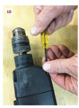
Reversing the process, the author uses needle-nose pliers to insert wires into their slots (7). Checking against the photos he had taken earlier, he repositions the switch and makes sure the wires are routed through the handle without being pinched (8). Then he screws the handle back together (9) and replaces the screws from the chuck end of the tool (10).
