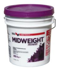
Companies such as USG and National Gypsum offer joint compound in a wide variety of weights and formulations. A few examples from USG are shown above: All-Purpose compound on the left can be used for embedding tape as well as for finish coats. Plus 3 is lighter weight and is for finish coats. Midweight is between the two and can be used for both taping and finish.
