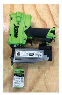
Light, powerful, well-designed, and cordless, the Grex 23-gauge pinner delivered on site and in the shop.
