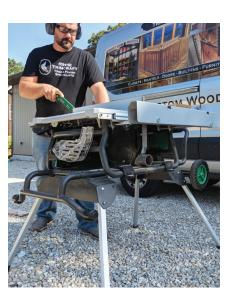
Metabo HPT's C3610DRJ cordless 10-inch table saw is built on the company's corded platform. At 5,000 rpm, the saw can handle the hardwood and plywood the author works with, and he gives the outfeed support bar high marks. The optional folding stand bolts to the saw and has locking legs.
