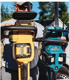
Both chain saws have the power to slice through framing lumber (top). The DeWalt gets it from one 60-volt battery; the Makita, from two 18-volt batteries.
