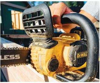
The Makita XCUO3PT1 18V X2 LXT 14-inch chain saw (above left) and DeWalt DCCS670 60V Max 16-inch chain saw (above right) both feature chain tensioning and bar tightening knobs for toolless chain adjustment. The Makita saw weighs 11.5 pounds (with two 18-volt batteries), while the DeWalt saw weighs 9.4 pounds (with a single 60-volt battery).
