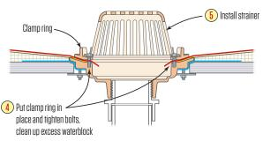
Common flaws in roof drain detailing allow leaks between the membrane and the drain body, and leaks between the drain body and the drainpipe. To avoid this scenario, the author recommends using a clamp-type drain that locks the membrane into the drain body. Watertight pipe connections are also crucial for preventing water from leaking into the building.
