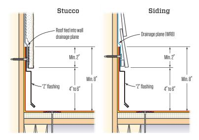
To tie the roofing into stucco or lap siding, the author recommends a "Z" flashing that laps under the weather-resistive barrier.
