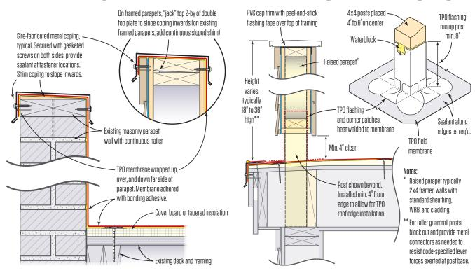
When roofing wraps up and over the top of a parapet wall, waterproofing the coping or trim is less critical. For optimum drainage at the roof's lowest edge, the author prefers a parapet raised on posts as shown above, with the post base wrapped in membrane. The tops of parapets should be shimmed for slope to prevent standing water from collecting.
