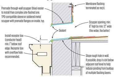
Drain receptors (conductors) are best positioned an inch or more below the scupper outlet so that clogs won't create leaks into the wall or ponding on the roof. Scuppers should be pitched to the outside.
