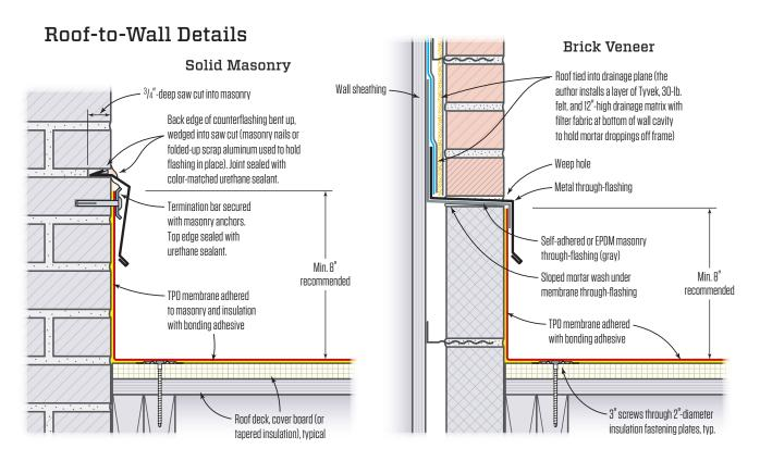
For solid masonry, the author recommends running the membrane 8 inches up the wall. The membrane is secured at the top with a termination bar and counterflashed.
