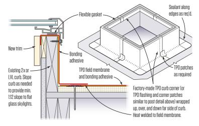
Preformed skylight curb corners help with wrapping membrane up and into the skylight curb. Skylights should be gasketed to block the intrusion of wind-blown water.
