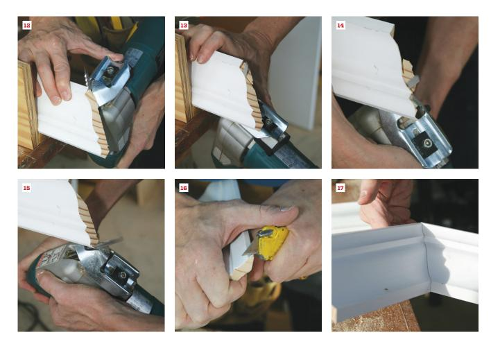
A coping foot mounts on a jigsaw in place of the footplate. The top three photos (12-14) show a typical sequence. For a mitered look, cut the angled sliver (15) and make a relief cut in the mating piece (16) so the two sides fit together (17).
