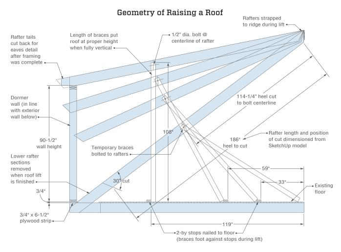
The author used SketchUp to plot the rotation of the roof from the existing pitch up to the pitch of the dormer roof. The program helped determine where the rafters needed to be cut. It also gave the crew the length and position of the temporary 2x4 braces, along with the locations of the floor stops to foot the braces as the roof hinged into position. When the braces were tight against the final stop, the dormer roof was at the proper height.
