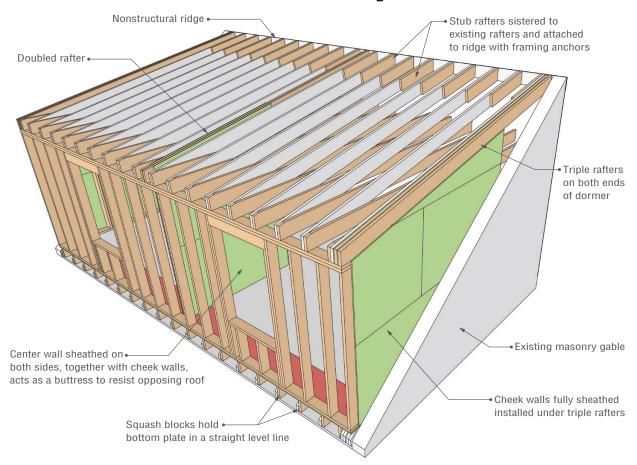
The crew framed the dormer using SketchUp to work out the details. Cheek walls at the ends of the dormer and a wall in the center of the dormer act as buttress walls. With continuous sheathing, they resist the thrust of the opposing roof, preventing the ridge from sagging, and eliminating the need for a structural ridge. At the ridge, stub rafters cut to the dormer roof pitch were sistered to the existing rafters. Framing anchors were used throughout to achieve the engineered specifications.
