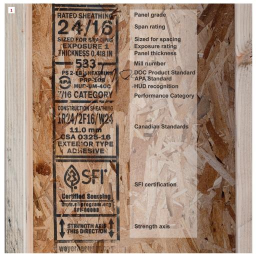
The panel stamp on structural OSB and plywood reveals key details. These are the ones you need to understand for shear walls: Panel grade: For walls, look for a "Rated Sheathing" designation.
