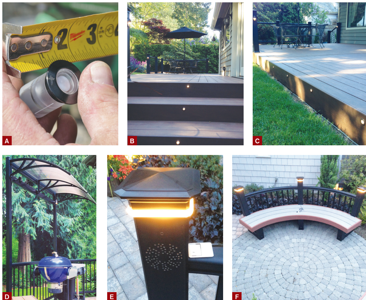
Figure 3. Measuring less than 1½ inches in diameter, small puck lights (A) are ideal for providing practical lighting in stair risers (B) and accent fascia lighting (C). When designing a system, be sure to provide task lighting to illuminate specific areas, such as dining tables and grills (D). Post-cap lighting adds both safety and style to outdoor areas (E, F).
