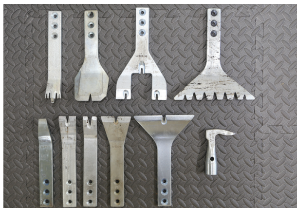
The salvage blade is useful for stripping siding (above left). Other blades include (above right, top row) finish nails; salvage; decking; 8-inch; and (bottom row) 3/4-inch; 1 3/4-inch; spike puller; 3-inch; 6-inch; and buried nail-head puller.
