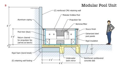
A rigging crew cranes a preassembled E-2000 Endless Pool unit into place (1). In the hilly Los Angeles neighborhoods where the author works, lots are tight and he often has to contend with existing retaining walls. SketchUp modeling was used to locate and design the support slab for the E-2000 preassembled unit (2) and the modular unit shown on page 51 (3).
