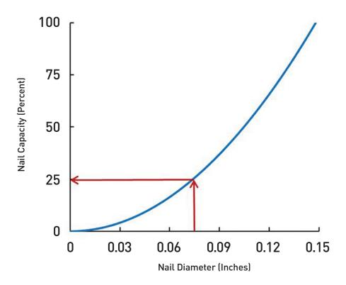
As red rust attacks the shank of a steel nail and effectively decreases its diameter, the design load capacity of the nail decreases accordingly. For example, if half the 0.148-inch diameter of a 10d common nail is lost due to red rust, the nail's design load capacity (90 pounds for wet use) would be reduced by 75%, with only 25% capacity remaining (22.5 pounds).
