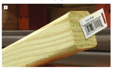
Typical of commercially available stress-rated pressure-treated 2x2 southern pine, this nominal 2x2 purchased at a lumberyard measures  $1^3/8$  inches by  $1^3/8$  inches, while the treatment tag reads 1.3125 inches by 1.3125 inches. Neither the measured nor the tag dimensions conform to the nominal dimensions of a 2x2 specified in the 2015 IRC.
