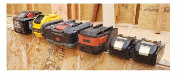
The high-amp batteries that drive these cordless saws come in a range of shapes and sizes. From left to right: Bosch; DeWalt; Skilsaw; Hilti; and Makita.
