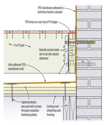
Where the roof deck is enclosed by a masonry parapet, ledgers can simply be bolted to the house framing and parapet to support standard deck joists (11). Ledger flashing is needed to keep water from penetrating the bolted ledger connections (12), which are typically specified by an engineer (see drawing, above right).
