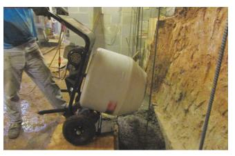
The compact MultiQuip MC3PEA Mix-n-Go mixer fits in the back of a pickup truck and—measuring only 24 inches wide—can be wheeled through a doorway (left). Mixed batches can be poured into a wheelbarrow or directly into a form (right).
