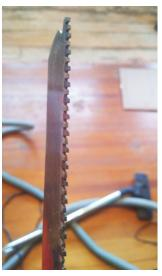
A recent job dismantling an old floor proved to be a good stress-test for the Diablo Steel Demon with "Amped" carbide (far left). Designed for cutting thick metals, this blade features wide gullets between the teeth (left). These help clear the metal flakes, which otherwise would build up between the teeth (as they do on the typical bimetal blade), creating lots of heat and slowing down the cut.
