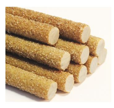
Glass FRP rebar is available in different sizes and grades for different applications. Shown here is Owens Corning's #3 Pinkbar Fiberglass rebar, which the company says is well-suited for flatwork thanks to its corrosion resistance, light weight, and ease of handling. Higher-strength fiberglass rebar for structural applications is also available.
