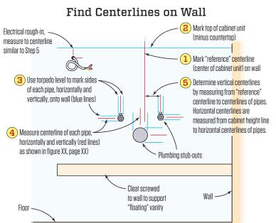
The existing conditions are precisely plotted on the wall (5). Layout marks include; cabinet "reference" centerline, vanity finish location, top of vanity, and plumbing and electrical centerlines (illustration, above).
