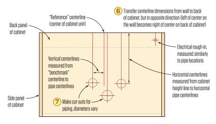
Layout information from the wall is transferred to vanity's back panel, but in opposite direction (illustration, above). Vertical centerlines measured from "reference" centerline to centerlines of pipes. Horizontal centerlines measured from cabinet height line to horizontal centerlines of pipes. A hole saw, going part way through the back panel, is used to make the cut-outs (6).
