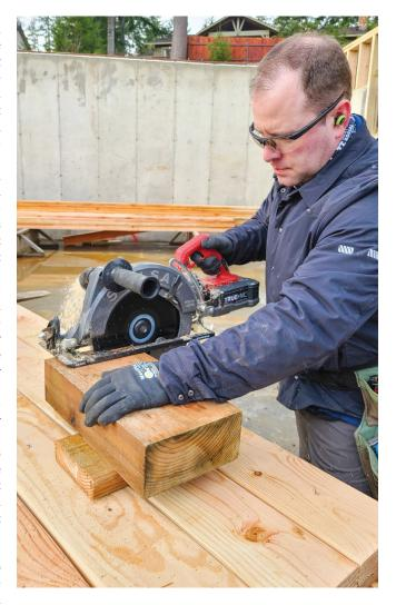
The Skilsaw Truehvl cordless wormdrive saw kit (model SPTH70M-11) offers a 311/16-inch depth of cut at 90 degrees, and 23/4 inches at 45 degrees. The kit comes with a single 5.0-Ah lithium battery, a quick charger, and a  $10^{1/4}$ -inch blade.
