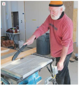
The right-handed author modified his saw, adding a left-hand cutoff switch to his saw as an ergonomic preference. The electronic blade brake, however, is integral to the factory switch (1). A carriage bolt head added to the outbound end of the fence allows it to glide on the rail friction-free (2). Commonly provided as standard safety equipment, a push stick is also easily custom-made and is an indispensable accessory to table saw use (3).
