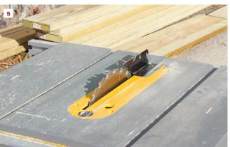
Power switches, shown here in a white circle, are deliberately configured to deter accidental activation while allowing quick, intuitive shutoff (4). A riving knife, aligned in the path of cut, holds the saw kerf open beyond the blade, helping to prevent pinching and kickback (5).
