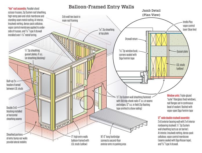
LSL members were used to balloon-frame the bump-out entry's 17-foot-high wall, while 2-by stock was used to infill shorter-length pieces such as trimmer studs, sills, and blocking. Sheathed areas on the south, east, and west walls helped provide lateral stability to these tall walls with big openings (the sheathing was nailed off per an engineer's specifications).
