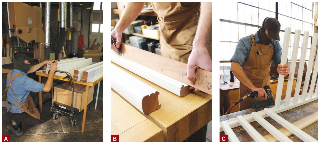
Figure 4. The author shaped and painted the railing parts in his shop (A), then used a story pole to lay out the baluster locations (B). He started assembly by pinning the balusters to the dado cut in the underside of the middle rail (C).
