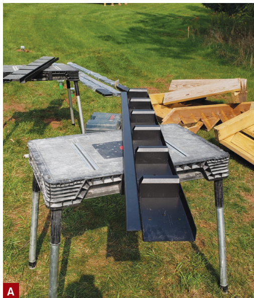
Figure 1. In the Evolution system, ledger brackets are screwed to the S-ledger, or fit into punched openings in the S-ledger without requiring additional fasteners (A). In comparison, an LGS ledger track has bent tabs for fastening the joists to the ledger (B) and requires five or more fasteners per joist-to-ledger connection. Evolution joists just slip over the brackets, and are held in place with a pair of screws per bracket (C).
