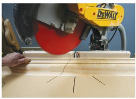
With the crown upside-down, measure its horizontal projection, then rip a gauge block to that width to use in setting the crown stop (left). The jig holds the crown molding in position when you're cutting the inside and outside corner miters needed to make a splice (right), and when gluing the joint together.
