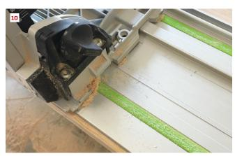
Friction strips are grippy, but track clamps ensure the line is held (6). Safety is enhanced by the fully housed saw blade (7), exposed only during plunge-cutting. Bevel cuts track along the rail edge without any adjustment to position. Here, the author miter-cuts 10-foot black walnut plywood using a 118-inch stock rail (8). A TSO guide rail square converts a rail into a 90-degree crosscutter (9). Without a vacuum hookup, sawdust quickly gums up the rail; constant clearing is needed (10).
