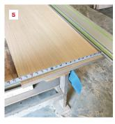
Track saws offer precise cutting of sheet goods (1). To avoid splintered veneer, first make a shallow pass (2), then recut at full depth. Black friction strips on the guide rail grip the cutting surface; the splinter guard edge (white, at right in photo) can drift and delaminate in use (3). The author bolsters the splinter guard with vinyl flashing tape to help prevent dislocation (4). For parallel cutting, measure to the back edge of the rail instead of to a time-worn splinter guard (5).
