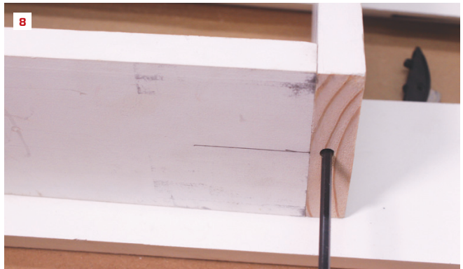
Available in a couple of sizes, the Clamex connector has a lever that is operated with a hex key, which allows the joint to be disassembled if desired (7). A small, 6-mm hole is required for access to the lever mechanism (8).
