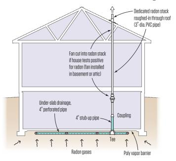
Crew members "tee" off the under-slab drainage piping (top left) and stub-up a 4-inch pipe into the basement (top right). A 3-inch pipe is run from the basement into attic and through the roof. A radon fan is cut in, if needed (illustration).
