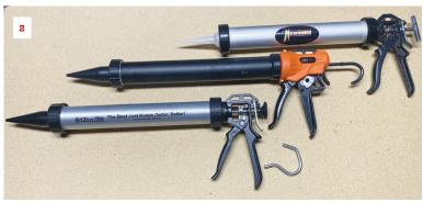
11-ounce guns (1): While basic "half-barrel" (orange) and "skeleton" guns (second from top) work, they're harder to use than professional-grade tools, which have a higher thrust ratio. The Irion-America gun (third from top) lets you switch between 12:1 and 25:1; the green Albion has a 26:1 ratio. The higher the ratio, the easier it is to apply more-viscous caulks. 20-ounce guns (2): All three "sausage" guns above are designed to hold sausage packs of sealant and have a 12:1 thrust ratio.
