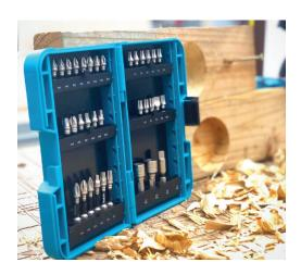
The author used Makita's Impact XPS bits during testing, which the company says last much longer than standard bits thanks to the carbon alloy steel used in their construction.
