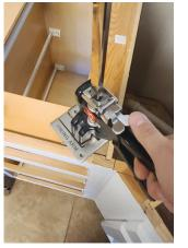
The Viking Arm can be used to both raise and lower heavy items such as cast iron sinks and cabinets with control and precision (above). The right trigger fully releases the tool; use the left trigger for controlled lowering action (left).
