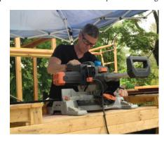
The Evolution R255SMS+ single bevel sliding miter saw has a maximum crosscutting capacity of  $11^3/4$  by  $3^9/16$  inches and weighs less than 34 pounds. The 14-amp motor has a soft-start feature and turns at 2,500 rpm.
