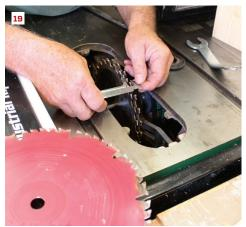
A caliper provides a quick and accurate check on tenon thickness (18). Using the caliper, the author adjusts dado thickness to match the tenon, adding washer-like proprietary thin metal shims between blades and chippers as needed (19).
