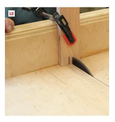
With an angle aligned to the sled's kerf, the author affixes a temporary fence for identical repeat cutting (10). In this repeat-cut setup, a fall-off block clamped to the fence greatly reduces the chance of post-cut jams between the fence and blade. The desired cut is measured between the sled kerf and block (11). Otherwise dicey cuts are performed safely and finger-free on the sled (12).
