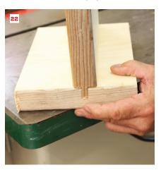
To avoid interference and inaccuracy, adjust the throat plate to be flush with the surrounding saw table (20). Set to depth, the dado blade cuts a wide kerf, sized to snugly fit the tenon (21). As a hedge against miscalculation, the tenon can first be run long, then trimmed to the precise depth of the slot. This joint is ready for glue (22).
