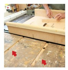
This crosscut sled uses both miter slots, left and right of the blade. To avoid distorting the kerf, the sled is best always used with the same saw blade (7). Accurate cuts are as simple as lining up the tick mark with the sled's kerf (8). The saw's miter slots are extended onto the outfeed table a fixed distance to prevent excess travel (9).
