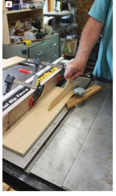
An application of ordinary paste wax minimizes surface friction and provides moderate rust protection to the cast iron saw top (1). Here, a hold-down clamped to the fence ensures a consistent depth of cut, with a fence board preventing lateral movement (2). A small steel ruler is more legible than a tape, whose hook partly obscures increments below the 1/2-inch mark (3).
