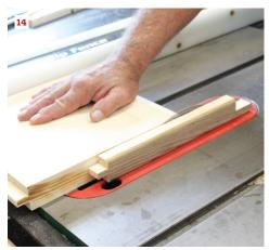
Use the right blade for the job: Dedicated crosscut (black), ripping (silver), and combination (red) blades are each designed for optimal perfomance in specific applications (13). Here, ripping a scrap of spruce with a sharp combination blade produces scorch marks on the lumber. A dedicated ripping blade's tooth configuration eliminates the friction responsible for the burn (14).
