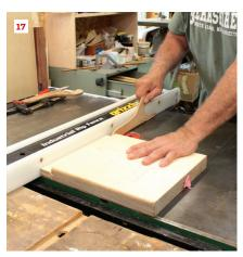
For this test-piece tenon, the author first adjusts for depth of cut against the layout line (15). To safely cut a tenon while preventing unwanted movement, clamp the workpiece to a simple tenoning jig (16). After readjusting the blade height, complete secondary shoulder cuts directly against the fence. To guard against violent waste-piece ejection, use a push stick to drive it past the blade (17).
