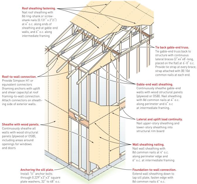
Illustration adapted by JLC from APA "Building for High Wind Resistance in Light-Frame Wood Construction Manual" [M310, 2015].
