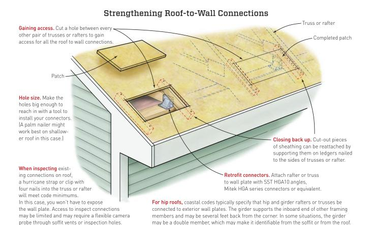
Retrofit framing. To minimize demolition of the roof edge, rectangular holes are cut into every other rafter or truss bay, and gusset angles are installed on each side of the hole. The cut-out can be saved and used to patch in the opening by securing it to scabs nailed to the side of the trusses.
