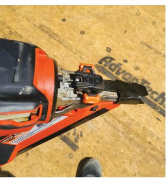
Paslode's cordless CFN325XP framing nailer is light at 7.2 pounds and compact enough to easily fit inside framing bays, making it ideal for installing blocking and other pickup work (left). It has an aggressive nosepiece that prevents the nailer from slipping when toenailing, and tool-free depth-of-drive adjustment (right).
