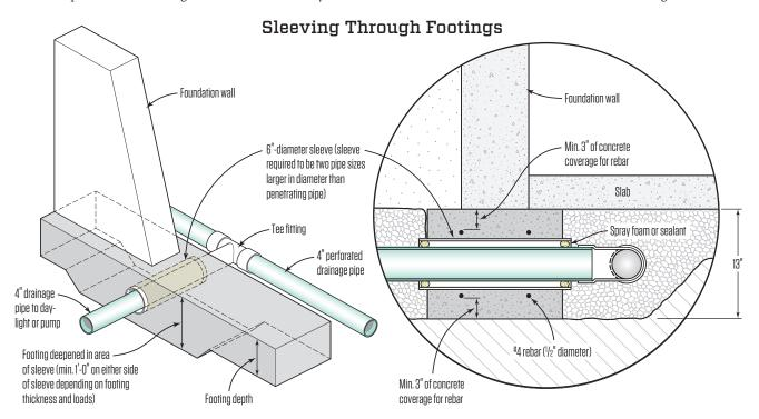
A protective sleeve that is two sizes larger than the pipe is required for any pipe that passes through a concrete foundation wall or footing. Depending on the size of the sleeve and the size of the footing, the footing may need to be deepened as shown to provide the required minimum 3 inches of concrete coverage for the rebar above and below the sleeve. The gap between the pipe and the sleeve should be sealed with spray foam or sealant.
