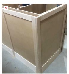
The author assembles the cabinet boxes out of  $^{3}$ /4-inch prefinished plywood (1), then uses a Lamello Zeta P2 biscuit joiner to cut slots for the Tenso P-14 biscuits that will be used to fasten the face frames to the boxes (2). Where the ends and backs of the cabinets will be exposed, such as for kitchen island cabinets, the author covers the plywood box with a separate frame-and-panel assembly, attaching it to the face frame with P-14 biscuit connectors (3, 4).
