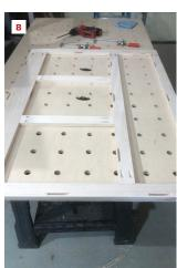
The author uses pocket screws and glue to assemble the face frames (5), then cuts the slots for the biscuits following the layout marked on the cabinet boxes (6). The two parts of the Tenso P-14 biscuit connect mechanically when fitted together but can be easily disassembled if needed (7). Holes bored in the plywood worktable make it easy to position the clamps used to securely hold the frame flat and square during assembly (8).
