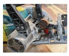
To test the new Makita XGT 40-volt rear-handle saw against its 36-volt predecessor, the authors made multiple crosscuts in a 14-inch LVL (1) and rips in a triple layer of 5/e-inch OSB (2) and compared results. Corking the dust port when it's not connected to dust extraction keeps sawdust from being deposited in a pile on the work surface (3).
