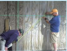
To test that the laser lines were perpendicular to each other, the author measured the diagonals between two equal sides, both on a floor (above) and on a wall (left).
