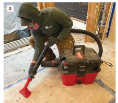
The Milwaukee M18 Fuel cordless wet/ dry vacuum is powered by a dualbattery motor head that can be fitted to a 12-gallon tank (1) or to smaller and more portable 6-gallon (2) or 9-gallon tanks. The 0930-22HD kit includes the 12-gallon tank and matching cart with a handle, along with a hose. extension tubes, a filter, and other accessories.
