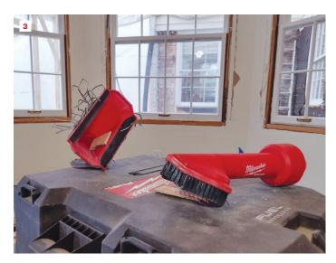
Crew members used several optional Air-Tip vacuum accessories that are available from Milwaukee, including a magnetic utility nozzle and a corner brush (3). When making cuts or drilling holes in walls, they found that the Air-Tip dust-collector attachment (4) was effective at scooping up debris.
