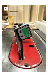
To determine octagonal facet, or "stave," dimensions, the author made segmented patterns from <sup>1</sup>/4-inch plywood (3). A calibrated digital angle gauge ensures precise beveling (4).
