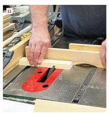
To bevel the tapered edges, the author raises the table-saw blade at  $22^{1}/2$  degrees into a sacrificial fence face, at the thickness of the stock (9). Decorative grooves are cut using a router table for tapered stock (10) and a dado blade in the table saw for parallel pieces (11).
