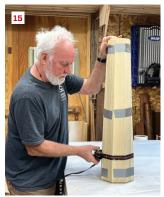
Tapered staves are aligned face down and edge-to-edge, taped together with duct tape (12), then flipped (13). Wood glue is applied to the open joints (14), and then the assembly is rolled up and band-clamped (15).
