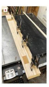
To cut the tapered column facets, the author uses a disposable jig on a table saw (5). Self-adhering sandpaper pads add friction (6). The first edge of all 32 pieces is cut, and the pieces stacked and marked to avoid accidental recutting (7). A tapered waste piece is added to the jig, establishing the second ripped edge (8).
