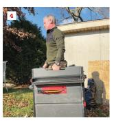
Skil's TS6307-00 10-inch table saw has sturdy fold-out legs (1). The author found that the paddle-off switch sometimes interfered with the smaller, push-button power-on switch (2). The plastic throat plate locks securely into place (3), and the saw is light enough for easy one-handed transport (4).
