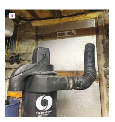
The Dust One air scrubber uses cyclonic technology, rather than filters, to separate contaminants from breathable air (1). Centrifugal force drives airborne particles away from the vortex and drops them into a collection bin at the bottom, which can be emptied by a HEPA vac when it fills up (2). In order to capture dust at the source, the flexible inlet extends almost 3 feet, bends in any direction, and stays where it's put (3).
