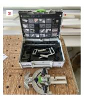
Fitting a Festool track-saw guide rail with the FS-WA angle stop and FS-WA-VL guide extension gives the saw the ability to make repeatable miter cuts at angles up to 60 degrees (1). The angle stop includes a pair of black positioning bolts that can be locked into the stop's T-track slots (2). The FS/2-Set includes the stop and other accessories and a Systainer (3).
