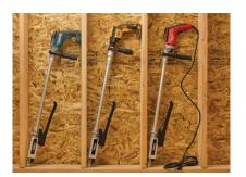
The PamFast cordless autofeed screw gun is powered by either Makita or DeWalt drivers (left) and comes with long and short extensions (below).
